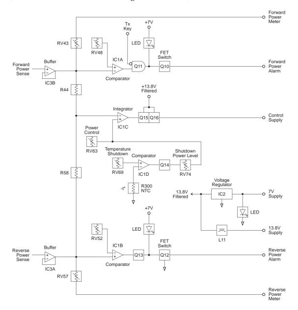
Figure 2.4 T828 Control Circuitry Block Diagram
