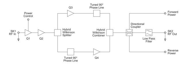
Figure 2.3 T828 RF Circuitry Block Diagram
