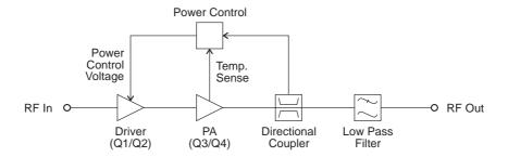
Figure 2.1 T828 High Level Block Diagram
